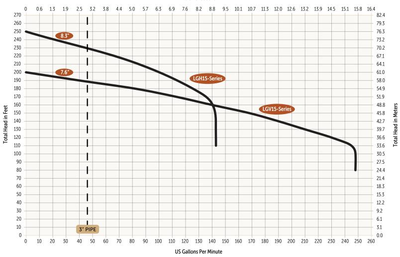
Pumps must operate within the proper range shown on the performance chart. It is the responsibility of the end user to ensure this requirement is met. Pumps operating outside the recommended range are prone to damage, excessive vibration, cavitation, poor efficiency, and may exceed nameplate amperage.
